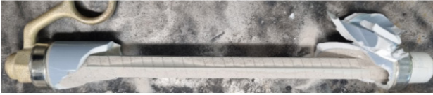
Fig. 4: Reformtech CLF fuse broken open to reveal a single fuse element [4]
