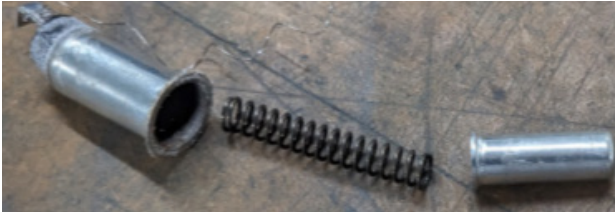
Fig. 10: Components of Reformtech full-range CLF triggering mechanism [4]
