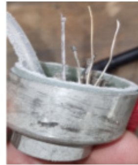
Fig. 6: Instead of the main fusing element, the bonding wires inside silicone tubes melted and broke the circuit after prolonged heavy arcing
