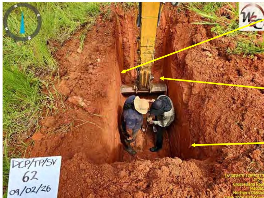
Photograph 10: Photograph indicating the dark brown Silty CLAY (topsoil) with rootlets and some quartz (shallow depth) and dark brownish orange Silty CLAY material which was extracted with excavator (TP 62) at deeper depth.
