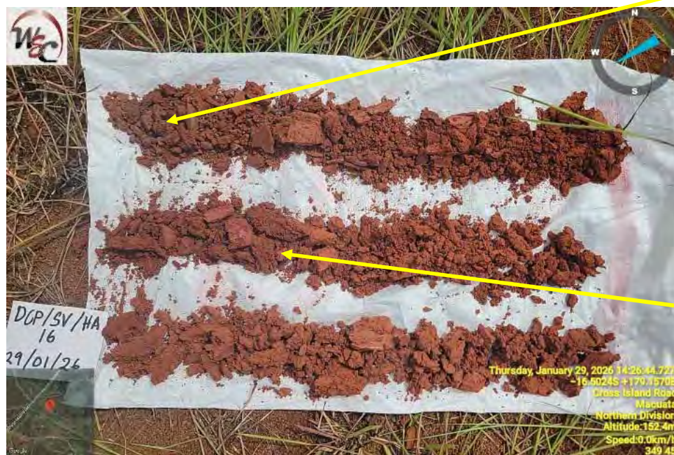
Photograph 7: Photograph indicating generally dark brownish orange Silty CLAY (Topsoil) (shallow depth), Silty CLAY with some rootlets and quartz which was extracted from Hand Auger (HA 16).
