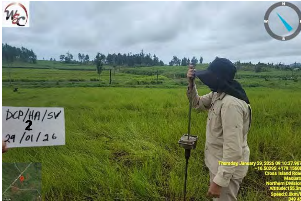
Photograph 1: Dynamic Cone Penetrometer (DCP) tests being carried out by WesEng Staff at Test location DCP/HA/SV 2 at EFL Seaqaqa Solar Farm Site.
