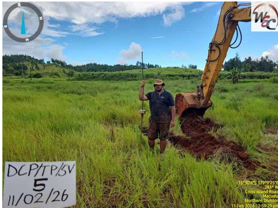
Photograph 12: Dynamic Cone Penetration tests being carried out by the Engineering Technician at Test Location DCP 5.
