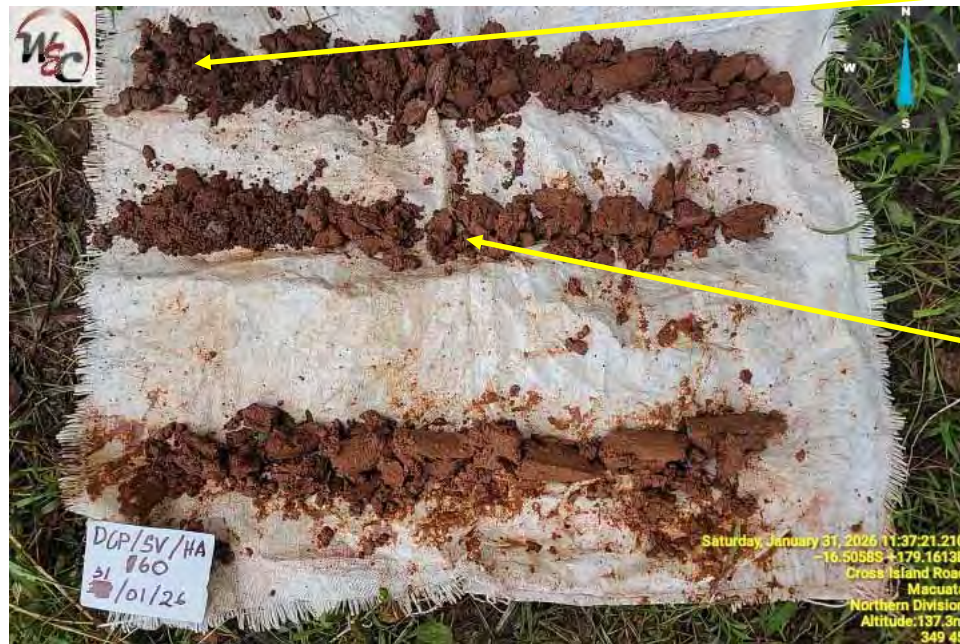
Photograph 8: Photograph indicating the dark brown topsoil to dark brownish orange soil profile with some rootlets and quartz which was extracted from Hand Auger (HA 60). The Silty CLAY was dark brownish orange and had trace of quartz at deeper depths.
