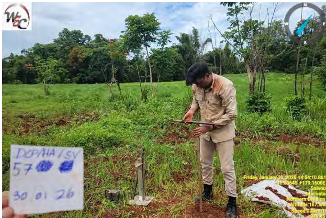
Photograph 4: Photograph indicating the Hand Auger tests being carried out at Test Location DCP/HA/SV 57 at EFL Seaqaqa Solar Farm Site.
