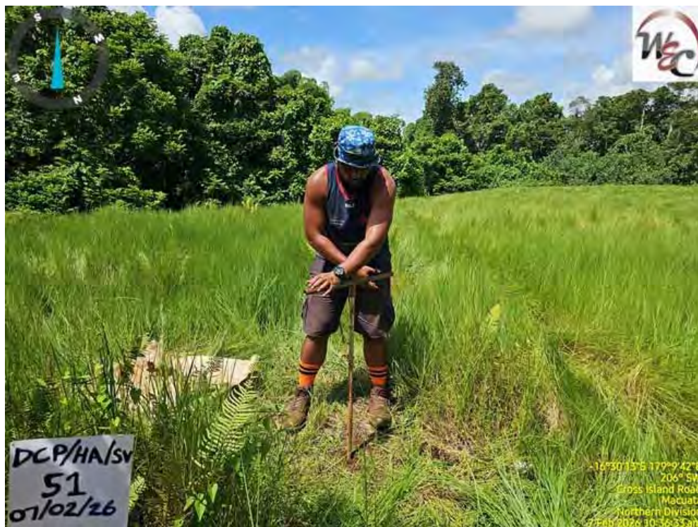
Photograph 5: Photograph indicating Hand Auger Borehole being carried out at Test Location DCP/HA/SV 51 at EFL Seaqaqa Solar Farm Site.
