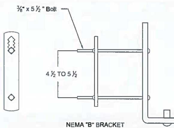
NOTE: NEMA B Bracket must be furnished with all Load Break and Non-Load Break cutouts.
