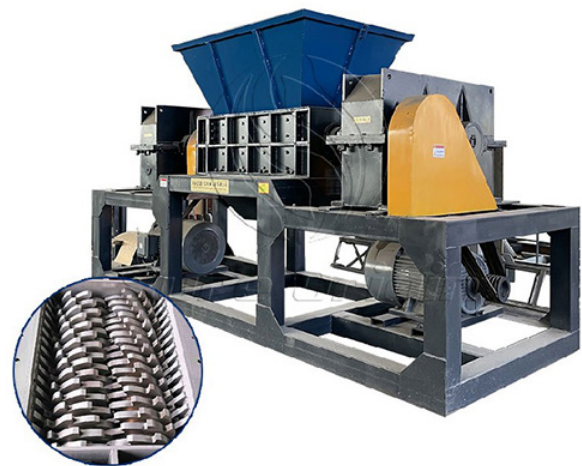
Figure 4 – Lithium-ion Battery Shredder (Source: Sure Origin Group).
