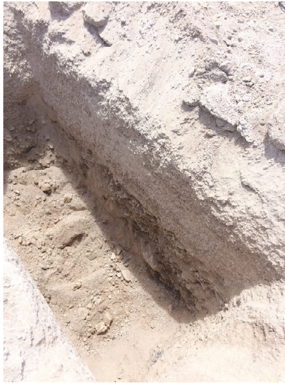
Figure: Typical excavated ground conditions in test pits
