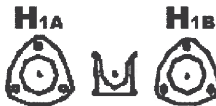
FIGURE 2. 13,800GRD Y/7970 V Loop Feed Bushing Configuration
