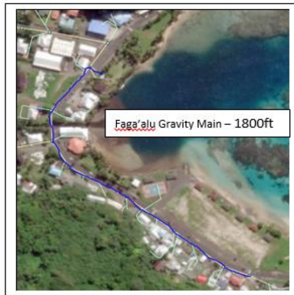
Figure #1 Location of Section that need Replacement
