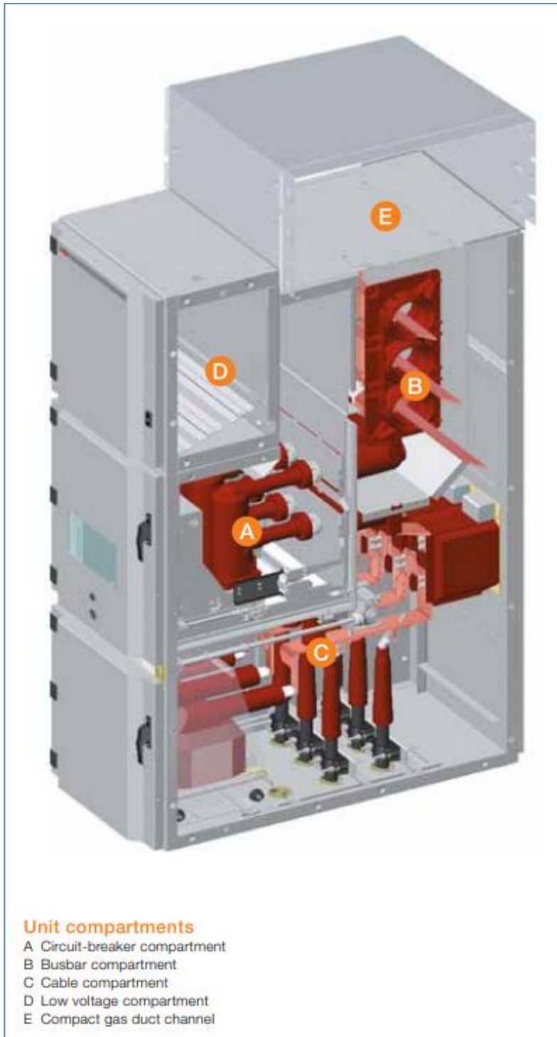
Figure 5-2 Switchgear unit compartments (indicative).
