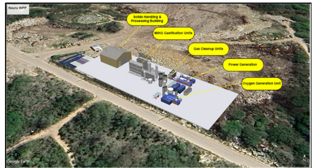
Figure 6: Concept 3D layout of Nauru WPP comprising one standard train of MIHG reactors, gas clean up equipment and gas engines and able to produce about 1 MWe net output.
