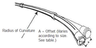
*NOTE:* Bent Pipes should be clearly marked along their length to avoid the possibility that they will be tapped in the future.
