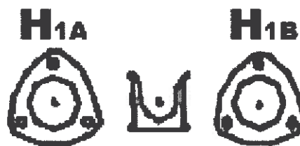
FIGURE 2. 13,800GRD Y/7970 V Loop Feed Bushing Configuration
