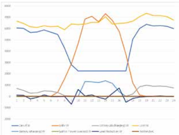
Figure 6- Optimisation of Solar, Battery and Load allowing for optimal load profile change to complement battery and solar usage.
