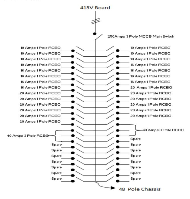
4. "FP DB - FUEL PUMP DISTRIBUTION BOARD"- name be printed on panel door
