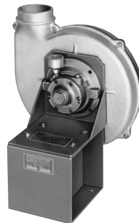
PB-9 with air motor. Cast aluminum blower with non-electric motor required to handle highly volatile substances at variable flow rates.
