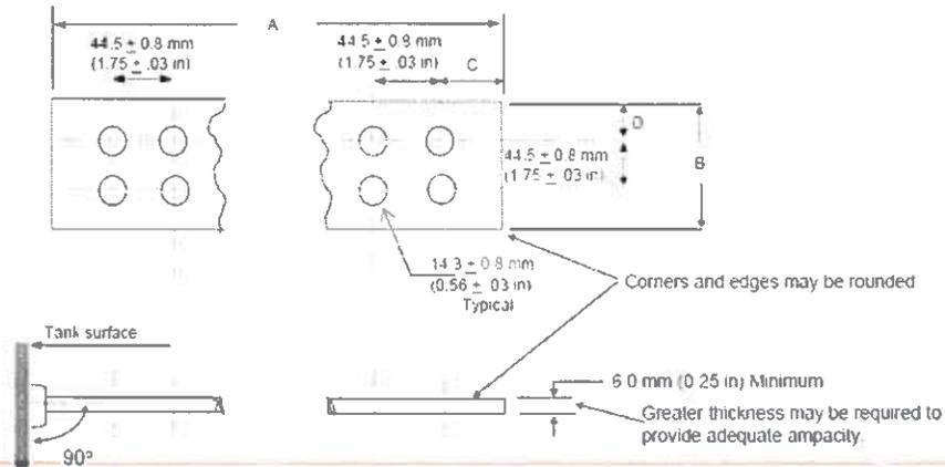
2. Low voltage terminals shall be plated for copper or aluminum cable terminations.
