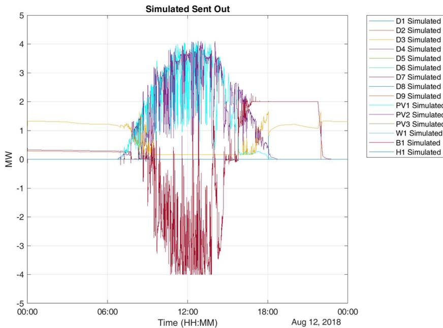
Case 5: Weekend (12 August 2018) - 12 MW of PV and 8 MW / 8 MWh battery on AGC
