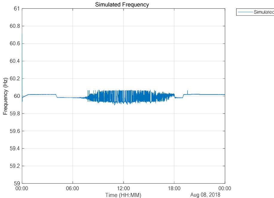
**Case 16: Weekday (8 August 2018) – 9 MW of PV and 2 MW / 2 MWh battery on AGC**
