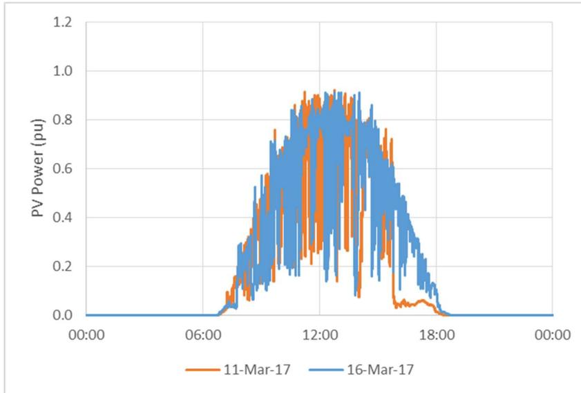
**Figure 3-15 Recorded 'normalised' one second PV output Base case 2 and 4**
