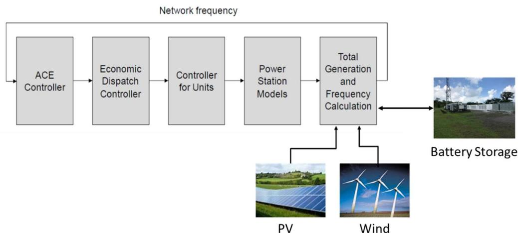
The studies undertaken in GDAT use original recorded generation, demand and frequency data from SCADA. The technical parameters for power plants such as ramp rates, network dynamics and frequency control capability are modelled. Additional constraints including spinning reserve, storage capability are also included. For Pohnpei, the studies are to determine the appropriate level of
