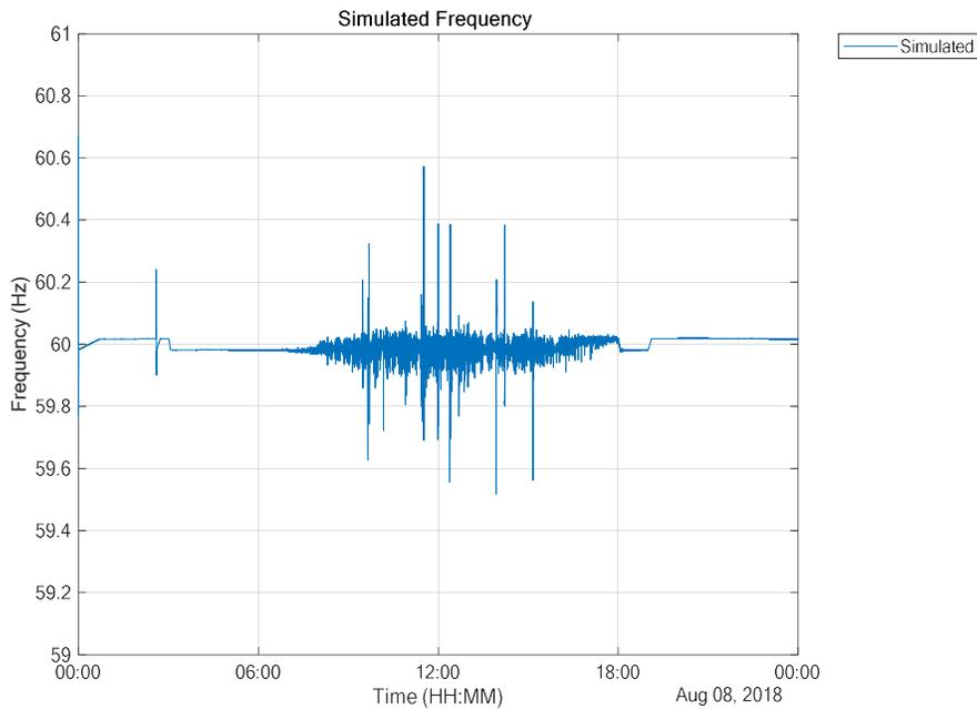
Case 14: Weekday (8 August 2018) - 3 MW of PV and 1 MW / 1 MWh battery on primary frequency control
