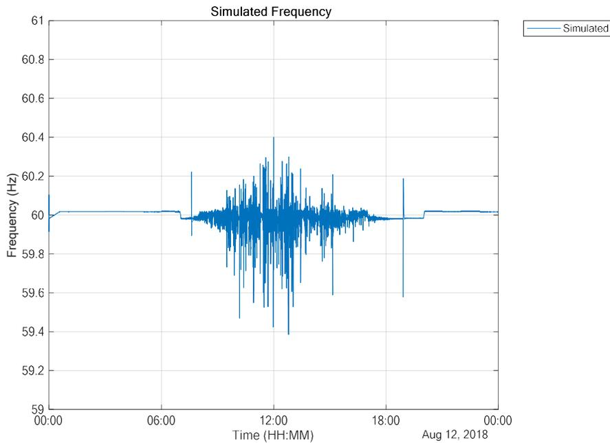
Case 2: Weekend (12 August 2018) - 3 MW of PV and 1 MW / 1 MWh battery on primary frequency control
