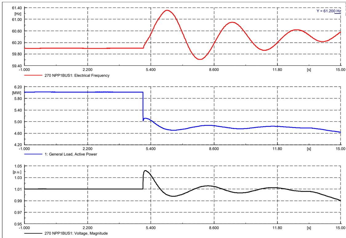
The frequency increases upon the loss of the Western feeder and marginally exceeds the limit of 61.2 Hz but it reduces quickly and remains within the acceptable bandwidth for the duration of the study. The voltage peaks at 1.04 pu but also remains within limits for the duration of the study.
