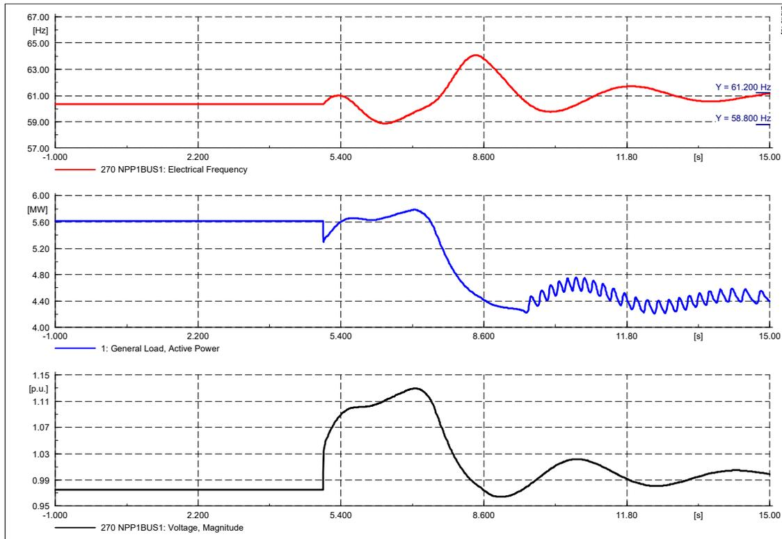
The loss of the Eastern feeder causes the system frequency to exceed the 2% deviation limit before returning to within the allowable bandwidth and settling. The voltage peaks at 1.13 pu and then reduces to within limits for the duration of the study.
