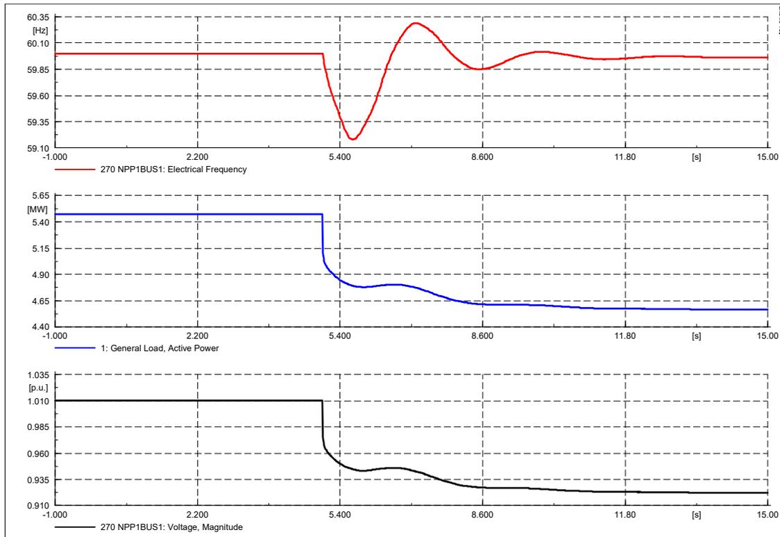
The frequency response of the system with this generation dispatch portfolio is improved and the frequency remains within the limits for the duration of the study. The voltage reduces to 0.92 pu following the event and stabilises there. This response is improved from the previous generation dispatch in Table 2-6 and no limits are exceeded.
