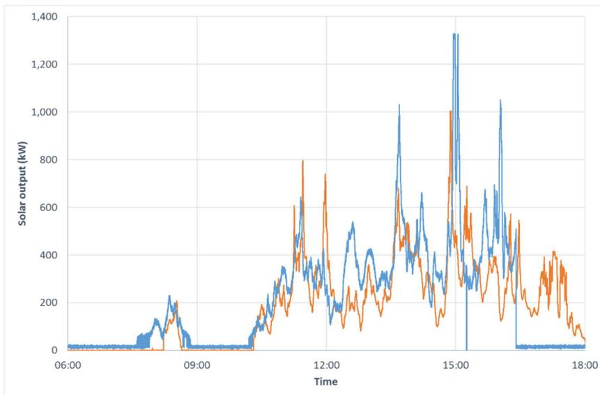
It seems that the two plants are exposed to the same cloud cover at the same time, but the combined output (Figure 3-3) shows there is not an exact correlation between the outputs of the two solar plants and the overall output is smoother than what would be obtained by doubling the output of the one farm.
