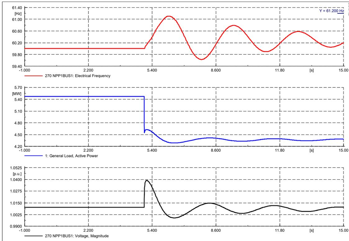
The frequency increases slightly upon the loss of the Western feeder but it remains within the acceptable bandwidth for the duration of the study. The voltage peaks at 1.04 pu but also remains within limits for the duration of the study.
