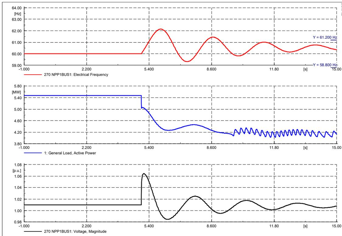
The loss of the Eastern feeder causes the system frequency to exceed the 2% deviation momentarily before returning to within the allowable bandwidth and settling. The voltage peaks at 1.06 pu but also remains within limits for the duration of the study.
