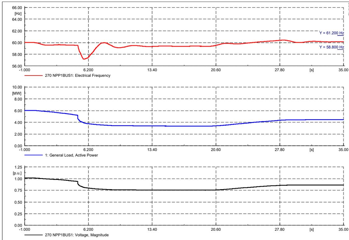
As the MW output of the PV generators decreases, the frequency decreases sharply to approximately 57 Hz, recovers then stays around 60 Hz for the duration of the study. The voltage reduces to 0.75 pu and voltage collapse in the system could potentially be the case when the PV generators ramp down. The simulation results indicate that in this operational scenario, the system is incapable of withstanding the drop and rise of PV generation within the given kW capacity and kW output level.
