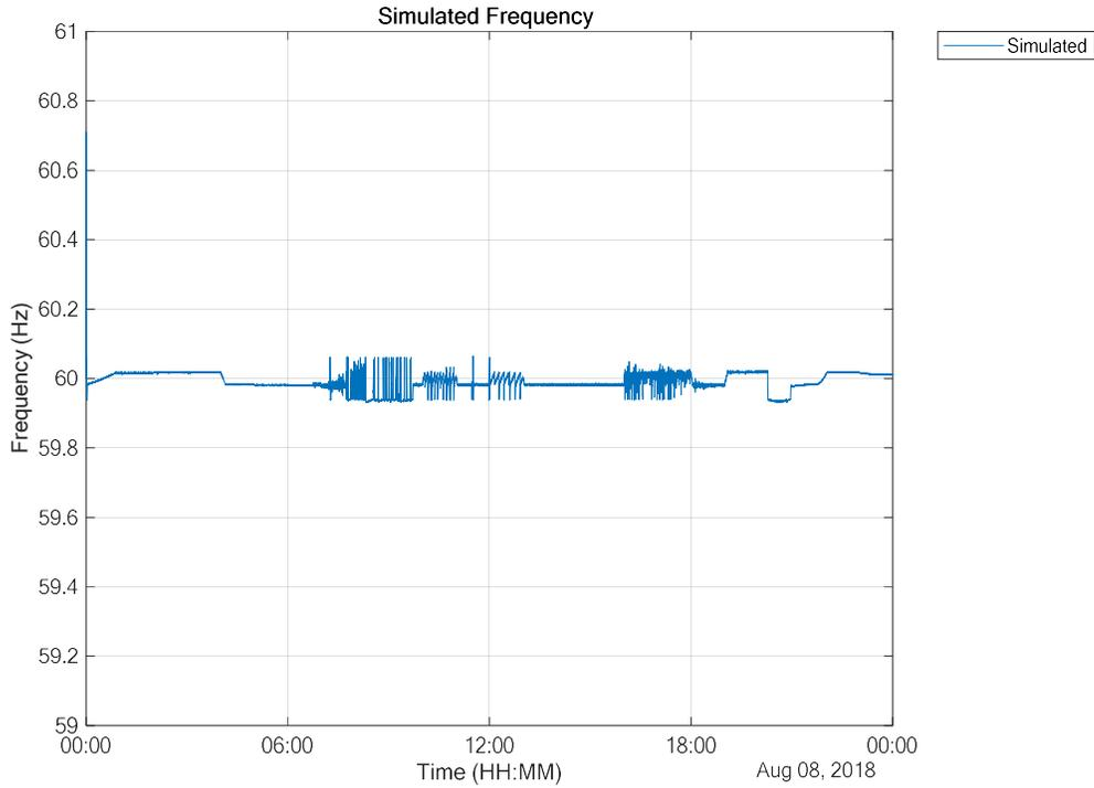
**Figure 3-58 Simulated generation output for weekday when 8 MW / 8 MWh battery provides both primary frequency control and AGC with 12 MW of PV. All diesel units allowed to go off.**
