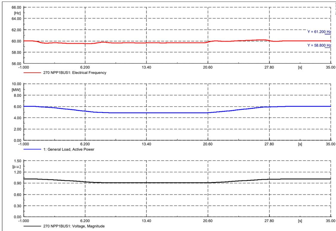
As the MW output of the PV generators decreases, the frequency decreases marginally and then fluctuates slightly around 60 Hz for the duration of the study. The voltage reduces to 0.9 pu when the PV generators ramp down which is just within the  $\pm 10\%$  limit for voltage. The simulation results indicate that with more conventional generators on line, the system is basically capable of withstanding the drop and rise of PV generation within the given kW capacity and kW output level.
