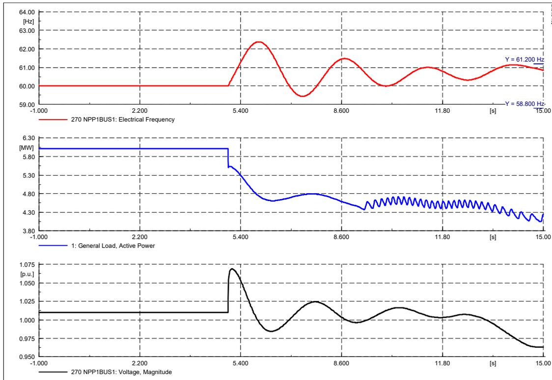
The loss of the Eastern feeder causes the system frequency to exceed the 2% deviation limit before returning to within the allowable bandwidth and settling. The voltage peaks at 1.07 pu but also remains within limits for the duration of the study.
