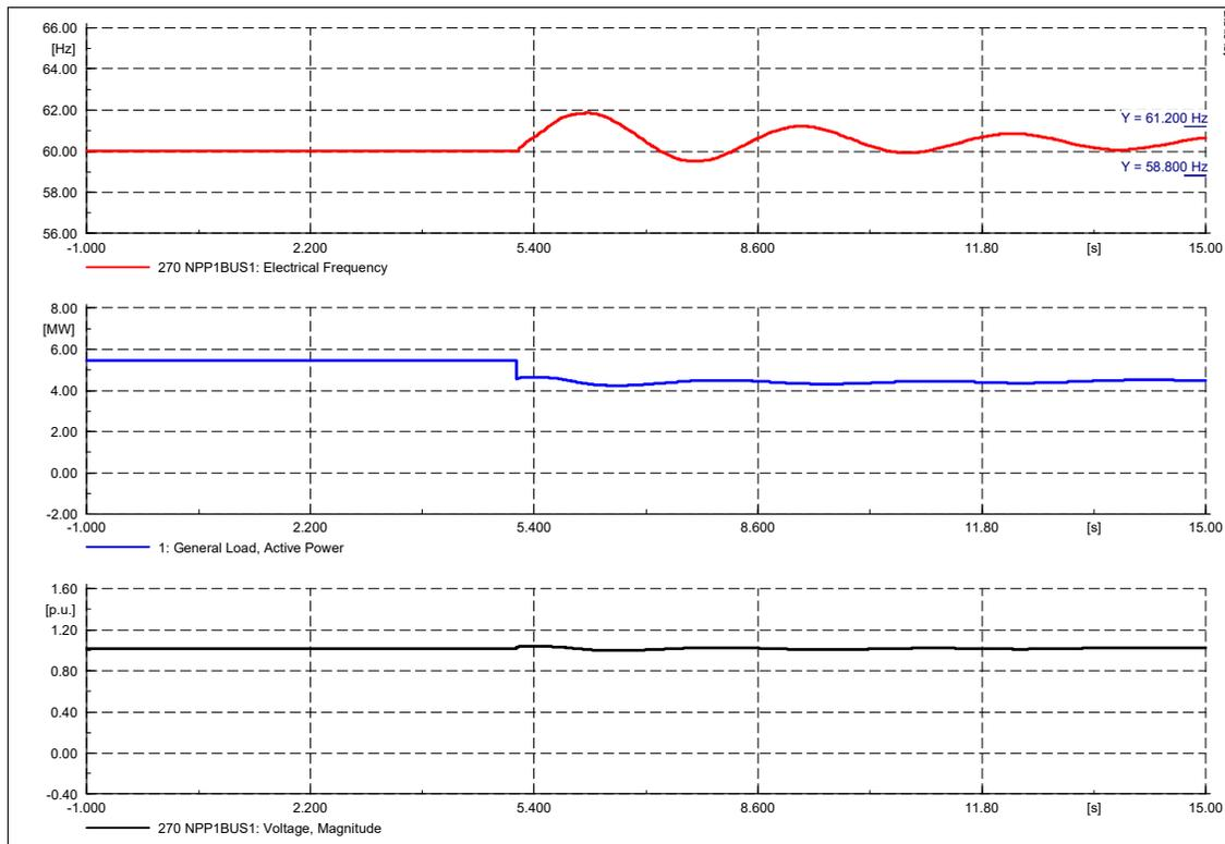
The frequency increases slightly upon the loss of the Western feeder and it exceeds the 2% deviation limit for around 1 second before returning to within the acceptable bandwidth and settling. The voltage remains within limits for the duration of the study.
