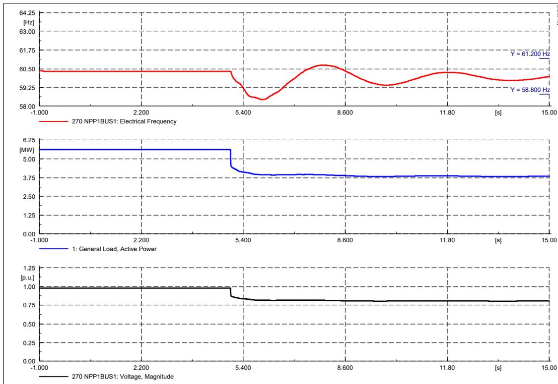
Upon the loss of the largest generator, the system frequency initially drops to 58.1 Hz which is outside the operational limits. The voltage drops to 0.8 pu which is in excess of the  $\pm 10\%$  limit for voltage. Voltage instability could thus be expected following the loss of the largest generator.
