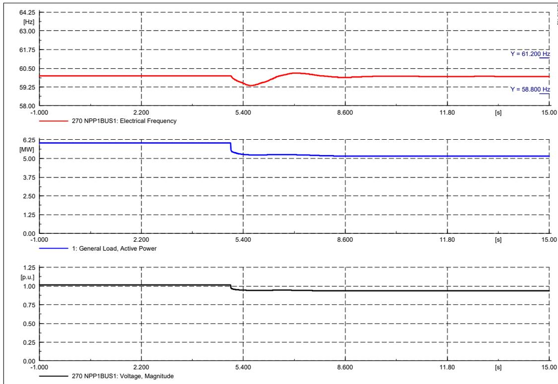
Upon the loss of the largest generator, the system frequency dips slightly but remains within limits and recovers quickly to nominal. The voltage drops to around 0.95 pu which is well within the  $\pm 10\%$  limit for voltage.
