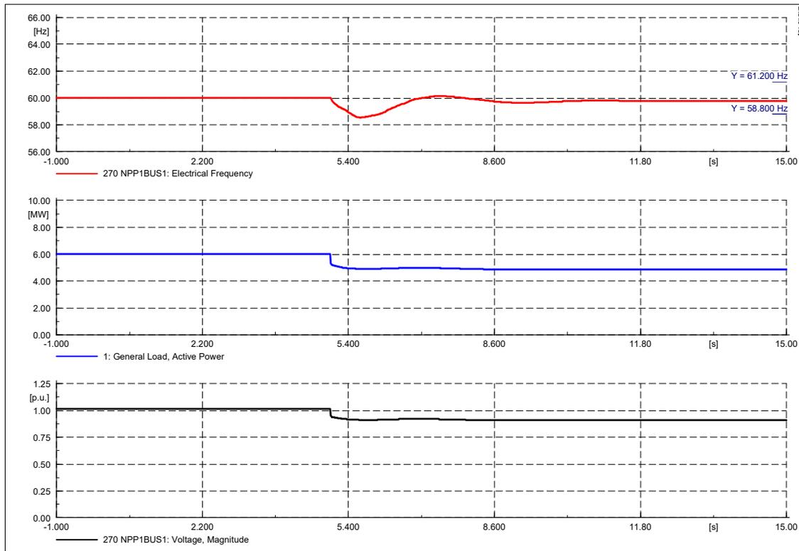
Upon the loss of the largest generator, the system frequency drops to 58.7 Hz which is marginally outside the 2% limit for frequency deviations, however this recovers quickly and there are no oscillations in the response. The voltage drops to 0.92 pu and remains steady at this value.
