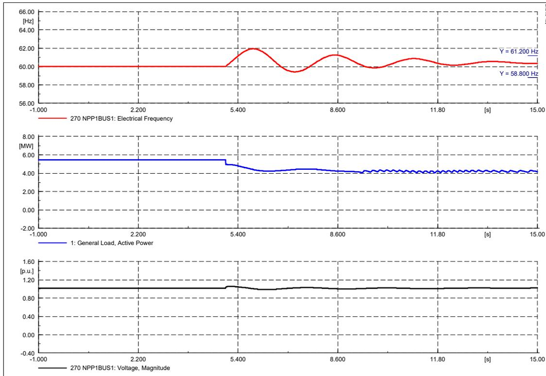
Similar to the Western feeder, the loss of the Eastern feeder causes the system frequency to exceed the 2% deviation momentarily before returning to within the allowable bandwidth and settling. The voltage remains within the limits for the duration of the study.
