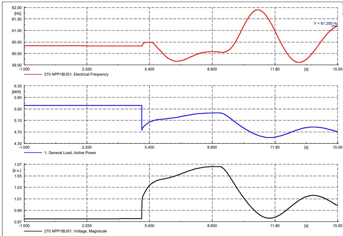
Upon the loss of the Western feeder the frequency swings upwards to almost 62 Hz and continues to oscillate for the duration of the study. The voltage peaks at 1.07 pu and has oscillations which mirror the frequency ones, however the voltage remains within limits for the duration of the study.
