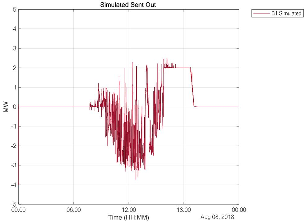
**Figure 3-52 Simulated battery charge level for weekday when 4 MW / 4 MWh battery provides both primary frequency control and AGC with 9 MW of PV.**
