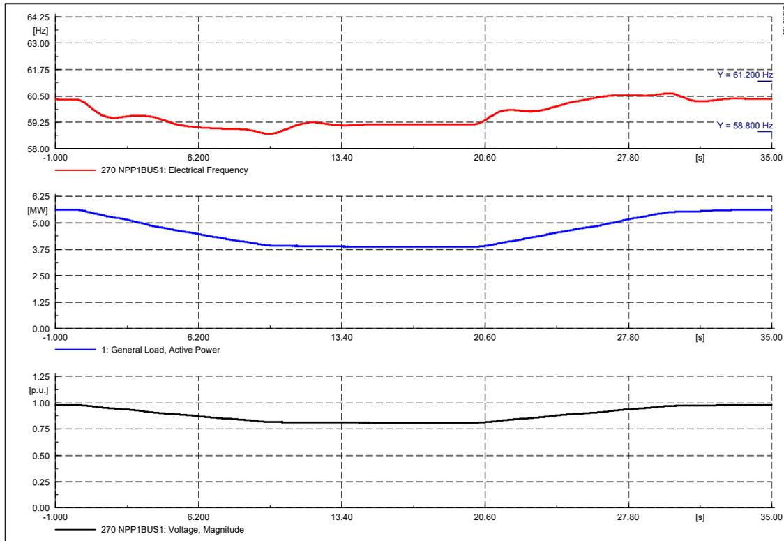
As the MW output of the PV generators decreases, the frequency decreases accordingly to slightly below 58.8 Hz and then steadily returns to nominal. The voltage reduces to 0.8 pu and the system may potentially experience voltage collapse when the PV generators ramp down. The simulation results indicate that in this operational scenario the system is incapable of withstanding the drop and rise of PV generation within the given kW capacity and kW output level.
