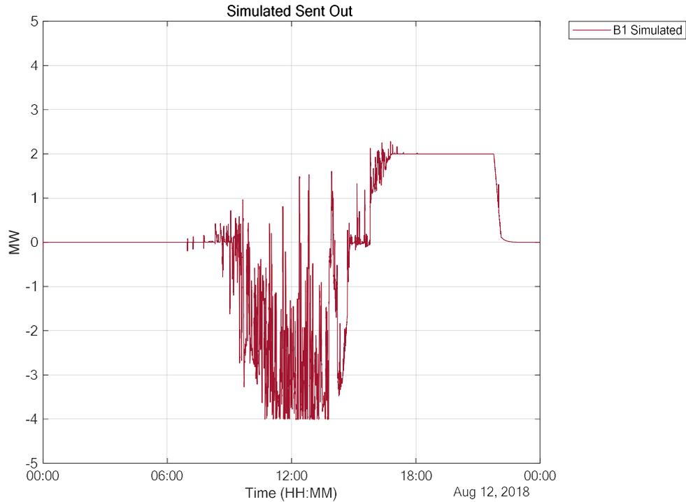
**Figure 3-27 Simulated battery charge level for weekend when 4 MW / 4 MWh battery provides both primary frequency control and AGC with 9 MW of PV.**
