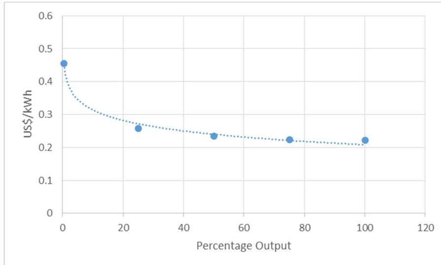
**Figure 3-12 Volvo diesel units cost curve**
