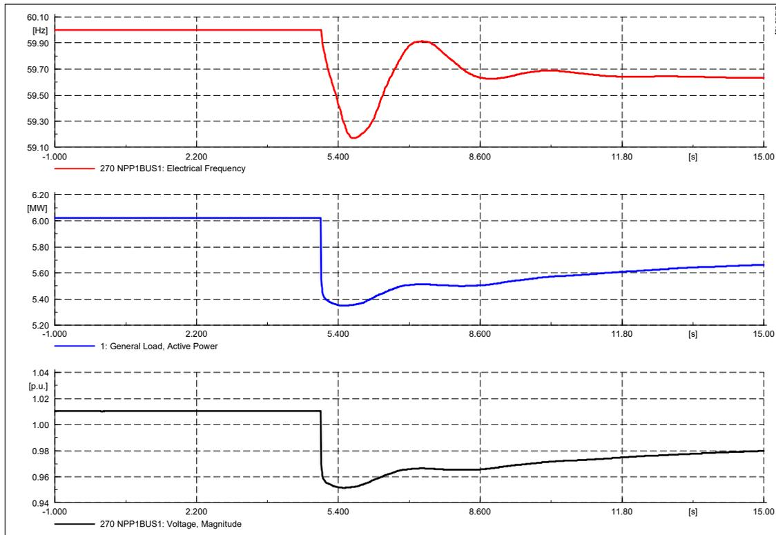
Upon the loss of the largest generator, the system frequency drops to 59.2 Hz which is within the operational limits. The voltage drops to 0.95 pu and increases steadily up to 0.98 pu.
