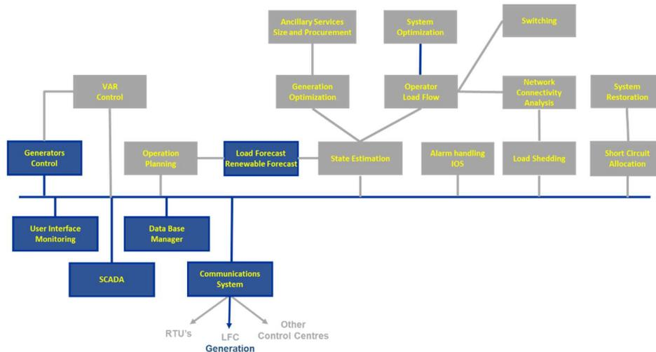
Battery and VRE control systems that have SCADA functionality also have the same capability to perform basic control functionality (such as open and close breakers), monitor system status (breaker
