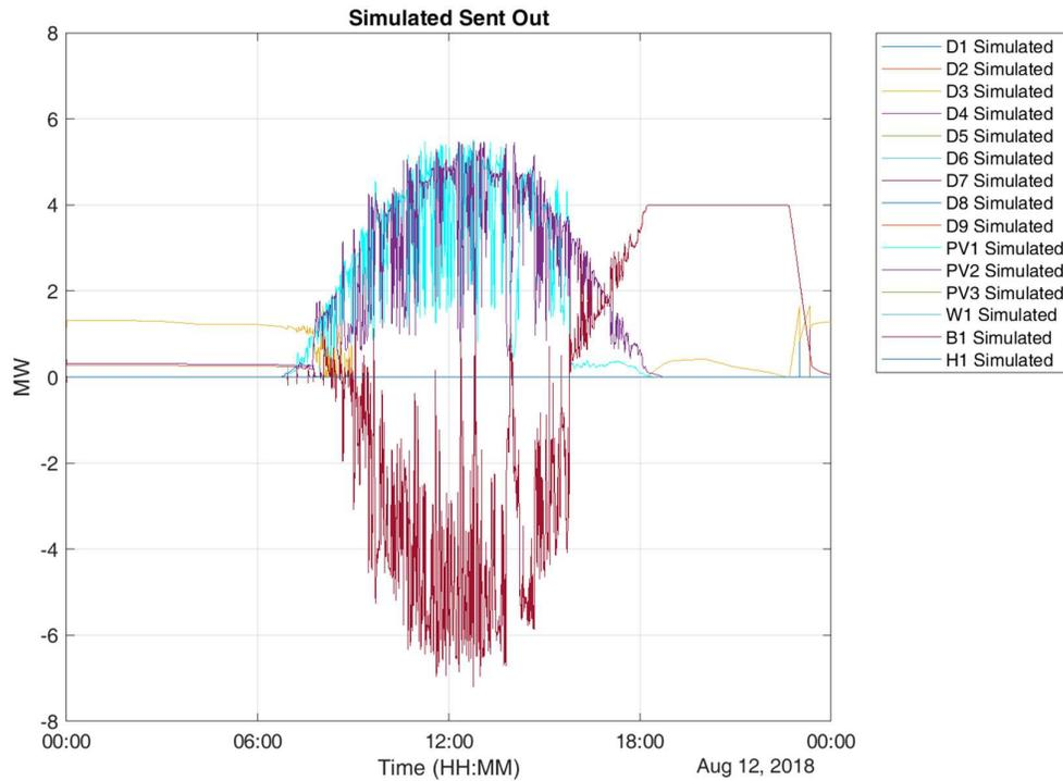
**Figure 3-33 Simulated battery output for weekend when 8 MW/ 8 MWh battery provides both primary frequency control and AGC with 12 MW of PV. All diesel units allowed to switch off.**
