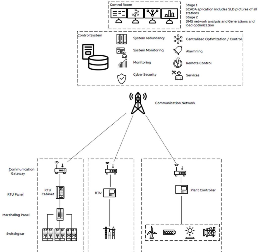
The conceptual design solution of the communication network is described in Figure 5-3.
