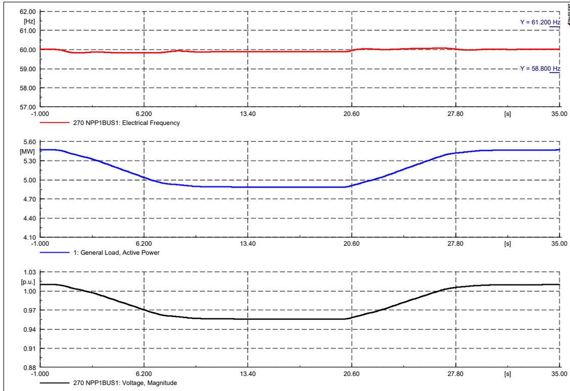
As the MW output of the PV generators decreases, the frequency decreases minimally and stays around 60 Hz for the duration of the study. The voltage Reduces to 0.95 pu and ramps up again to 1.01 pu as the PV generation increases back to 80% output. The simulation results indicate that in this operational scenario, the system is capable of withstanding the drop and rise of PV generation within the given kW capacity and kW output level.
