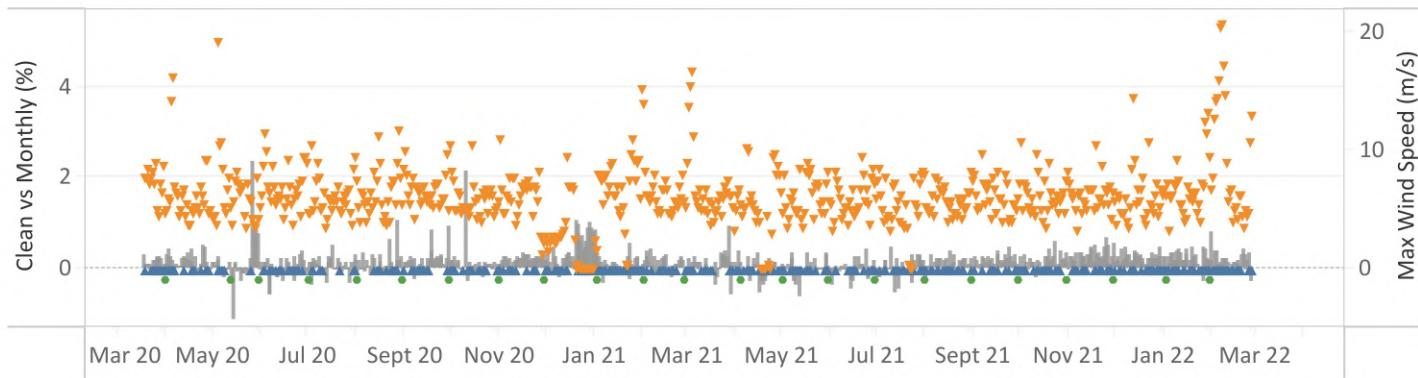
Figure 31: Soiling Measurement (Clean vs Monthly)
