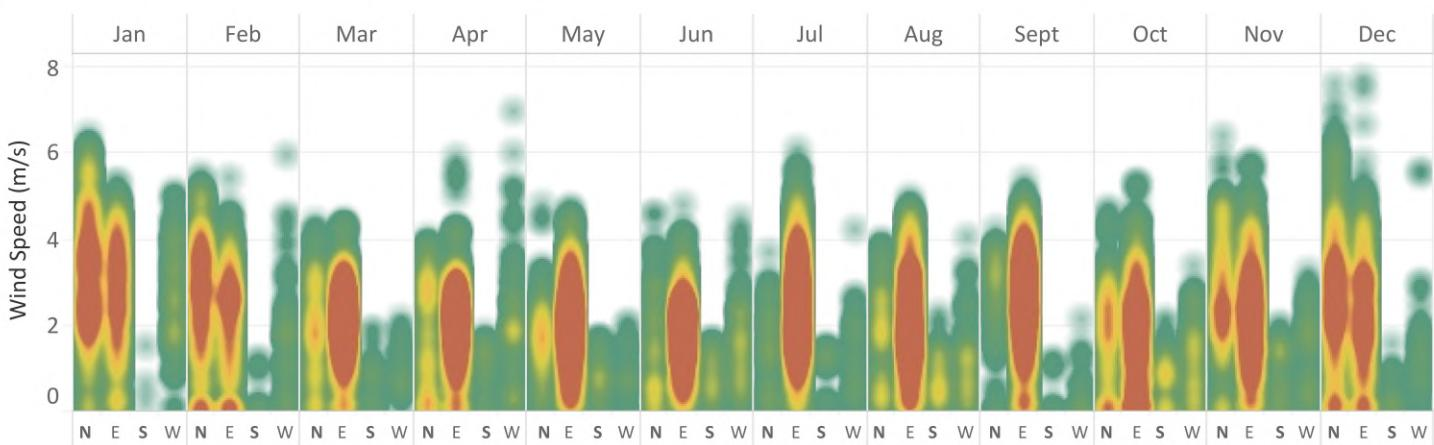
Figure 29: Hourly Wind Speed average compared to hourly Wind Direction
