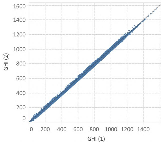
Figure 22: Comparison of GHI (1) and GHI (2) (YTD) ( $\text{W}/\text{m}^2$ )
