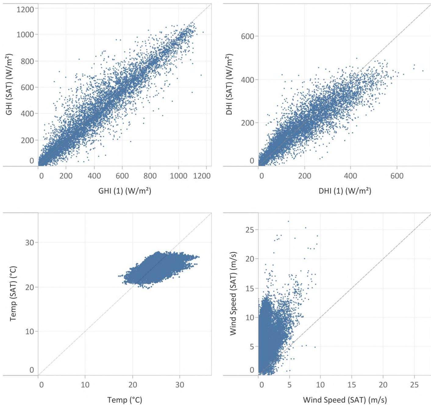
Figure 34: Ground measured data compared to satellite derived (Solargis) data
