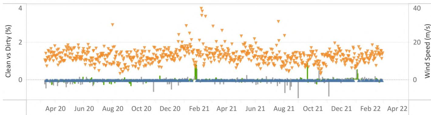
Figure 32: Soiling Measurement (Clean vs Dirty)
