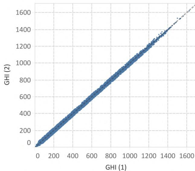
Figure 22: Comparison of GHI (1) and GHI (2) (YTD) ( $\text{W}/\text{m}^2$ )
