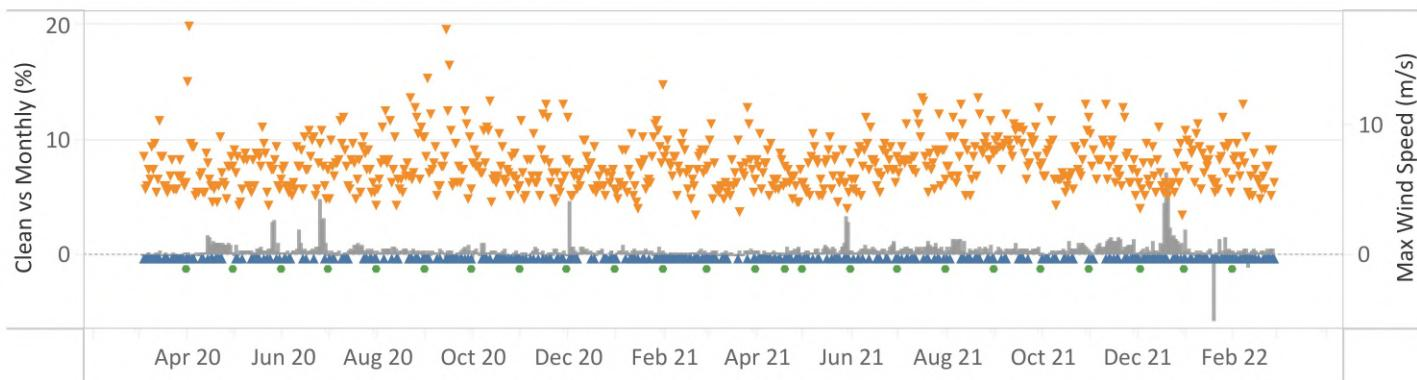
Figure 31: Soiling Measurement (Clean vs Monthly)
