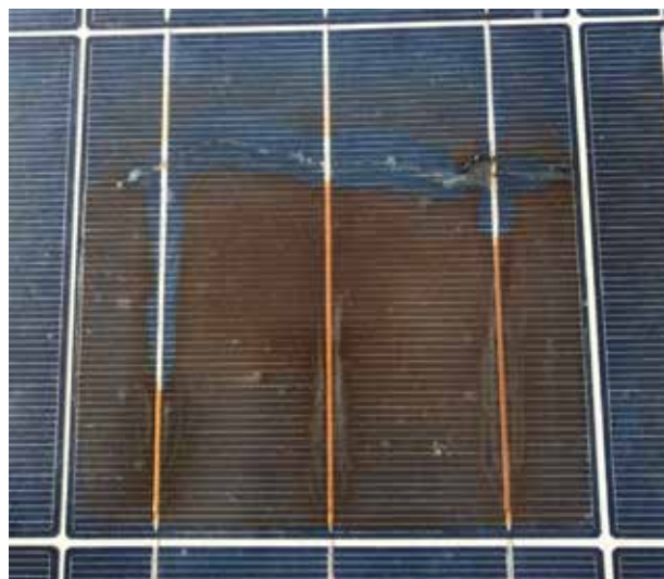
Figure 14 - cell degradation and hot spot from crack in module
