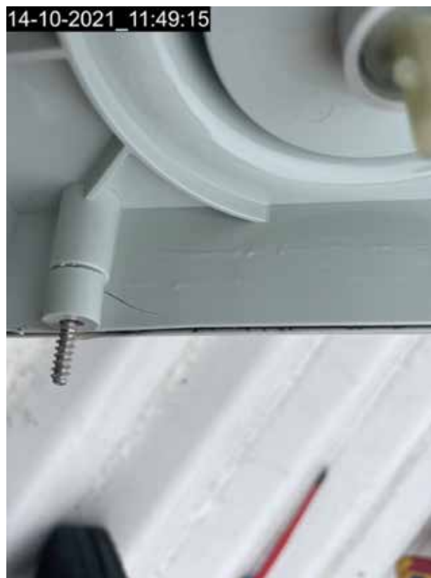
Figure 9 - An overtightened screw causing damage to the enclosure.
