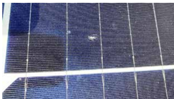
Figure 13 - evidence of damage on the front side of the module. The cracks are points of high resistance in the cell and can lead to hot spots.
