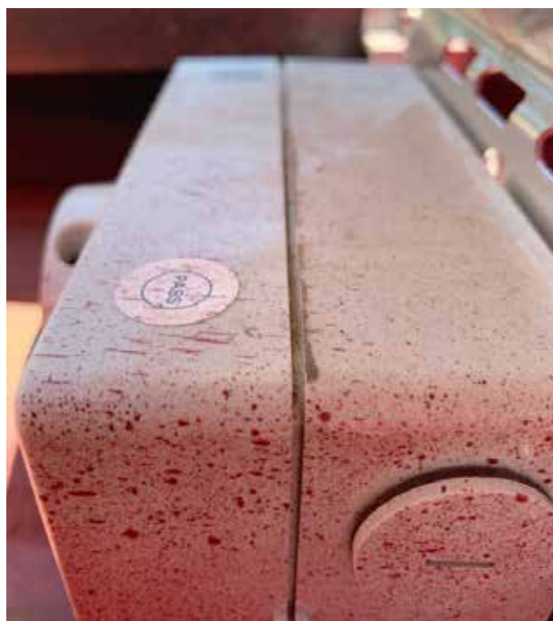
Figure 8 - loose screws causing inadequate sealing of the lid.
