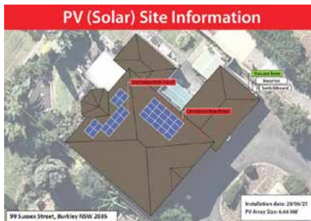
Typical solar system layout located at switchboard: see Appendix A5 in AS/NZS 5033:2021
