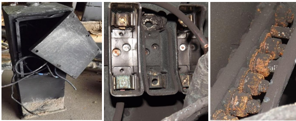
Fig. 2. Burnt plastic service pillar and its internals. Root cause - increased contact resistance and overheating of fuse contact; condensation and corrosion of contacts, including on Neutral-Earth bar
