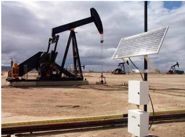
Solar-powered Remote Terminal Unit (RTU) at a pumping site using a Morningstar HazLoc-rated SunKeeper controller. Courtesy of SunWize
