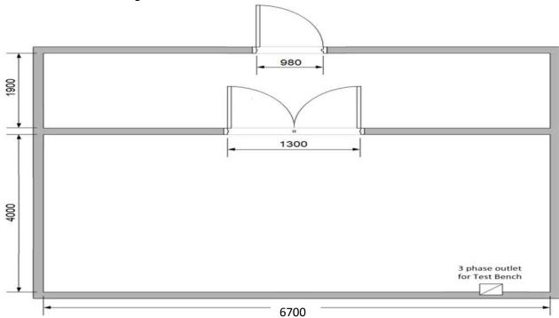
The dimensions of the **existing** meter test station are as follows
