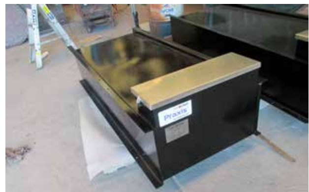
Completed generator base tank for Terra Cat
