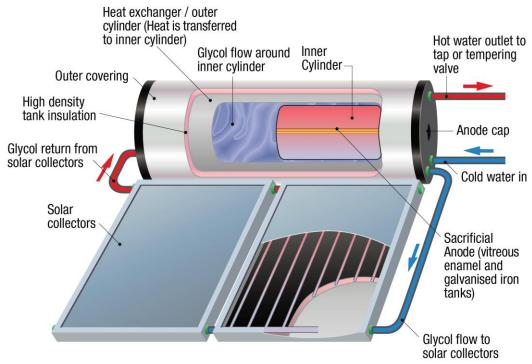
For sites having poor quality water supply, indirect systems would be useful in overcoming the build-up of calcium carbonate in the tank. The poor-quality water may contain sediment, which is any solid material carried by water, travels with the water through the pipes and into your home's hot water tank, causing an
