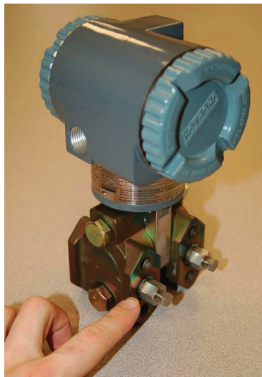
Figure 5: Typical Industrial Differential Pressure Transmitter With Heavy Duty Enclosure and Manifold Style Mounting Block. Can Be Used For Various Pressure, Flow and Liquid Level Measurements.
