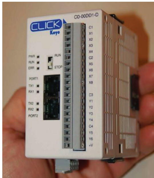
Figure 3: Typical Programmable Logic Controller CPU (Central Processing Unit) Module Showing Status Indication.
