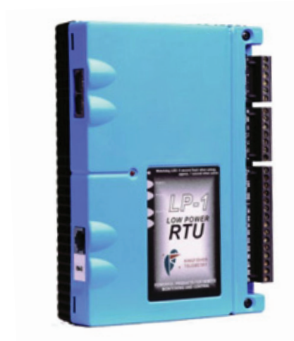
Figure 4: Typical Programmable Logic Controller CPU Module Showing Status Indication LEDs, Run/Stop Control Master Control Switch, Multiple Communications Ports and Digital Input/Output Points For Attachment Of Field Cabling. This CPU Module May (Like Most) Be Coupled With Additional Plug-In Modules To Expand The Available Digital, Analog and Communications Input/Output Capabilities.
