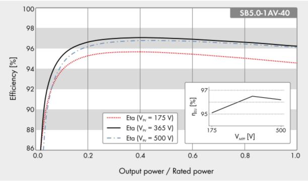
• This curve indicates that the inverter is above 96% efficiency for most of its operating range so using 96% would be good conservative figure.
