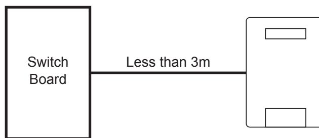
Figure 19: An ac switch-disconnector is not required - the distance between the switchboard and the inverter is less than 3m (10 feet) and the inverter is visible from the switchboard
