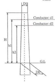
Pc: Design Load of Pole (kg) Pp : Pp=74 Wind Load of Pole (kg/m2)
