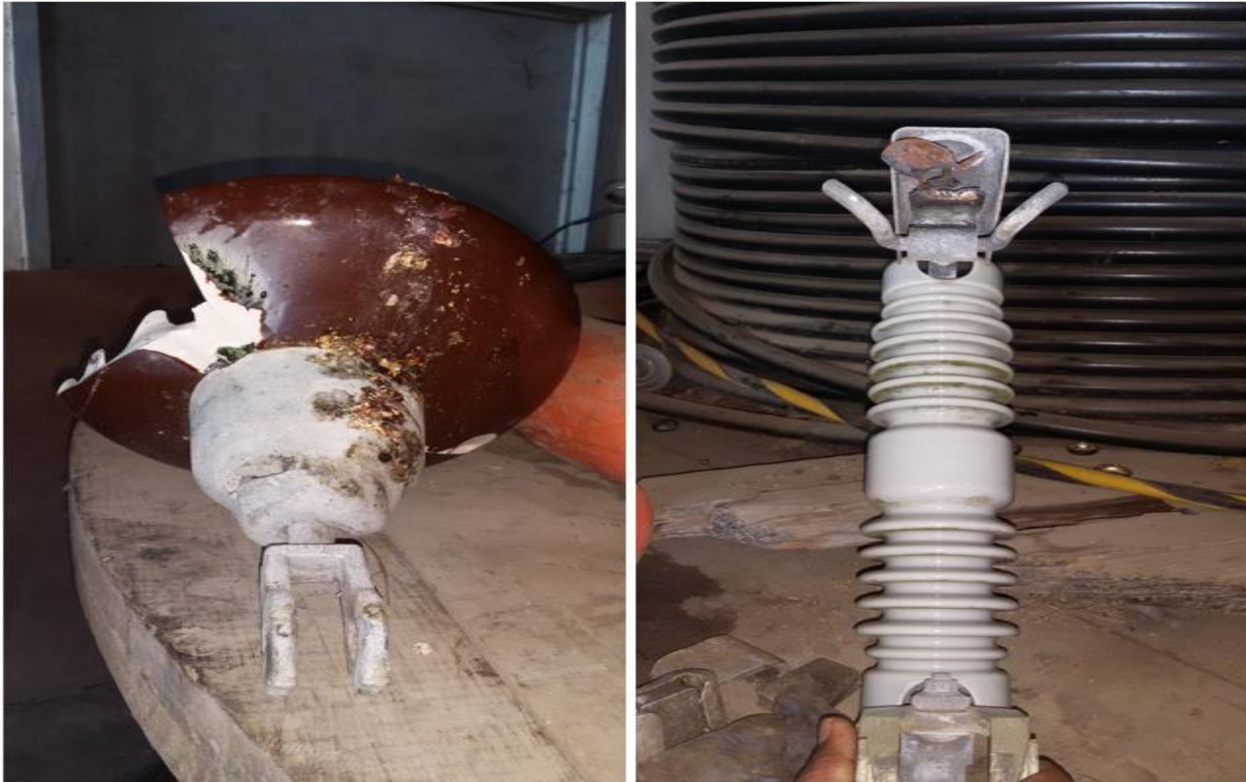
Figure 4: Unplanned Outage Works (Bat secretion causing short circuit on Disk Insulator & Old Hardware)
