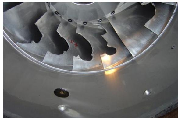
Figure 20 Unit 5 Runner Blade failure due to running of the unit outside operational limits 2012
