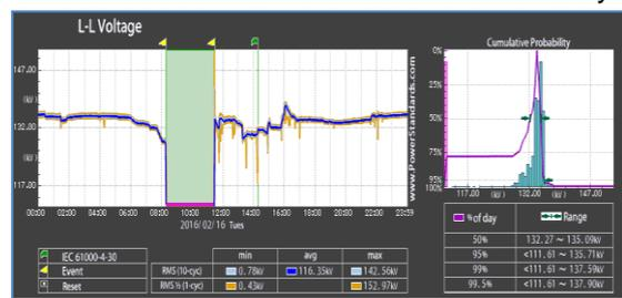
Figure 15 Voltage profile of L601 after an outage event 16/02/16
