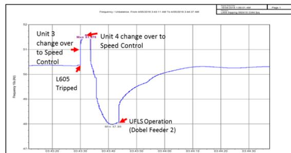
Figure 25 System Frequency during L510 fault
