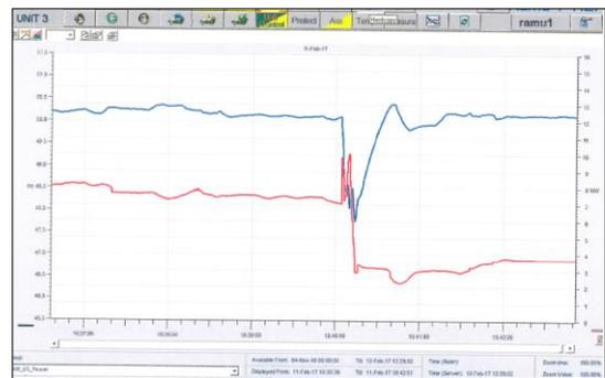
Figure 24 Response of Ramu1 Unit 3 to the Lae GT Tripping 11/02/17
