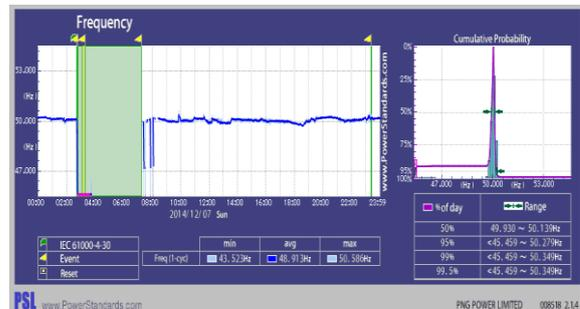
Figure 5 Ramu System frequency degradation 07/12/2014
