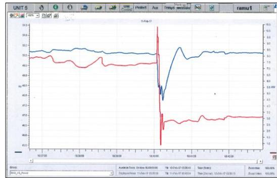
Figure 23 Response of Ramu1 Unit 5 to the Lae GT Tripping 11/02/17
