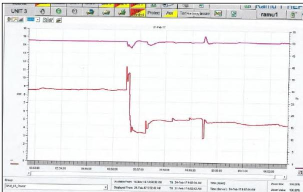
Figure 14 Assistance of UFLS in frequency stability in the loss of the L601 21/02/17
