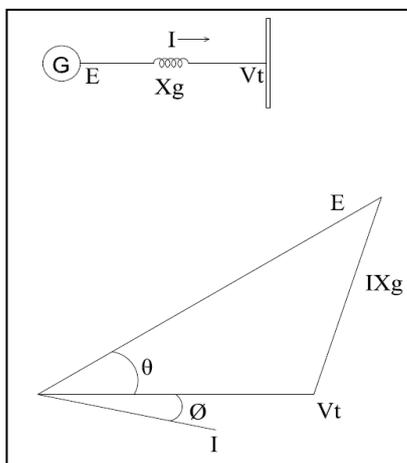
Figure 1 Synchronous machine vector diagram
