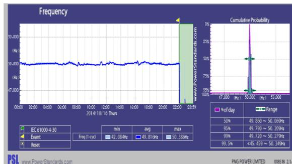
Figure 6 Ramu System frequency degradation 16/10/2014
