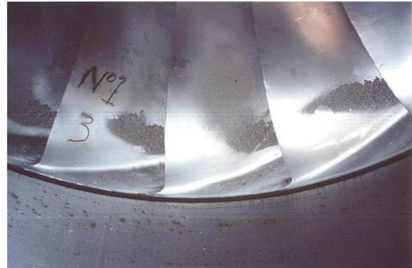
Figure 19 Ramu Unit 1 Cavitation Pitting 2012
