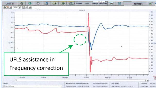
Figure 13 Assistance of UFLS in frequency stability in the loss of the Lae GT 11/02/17
