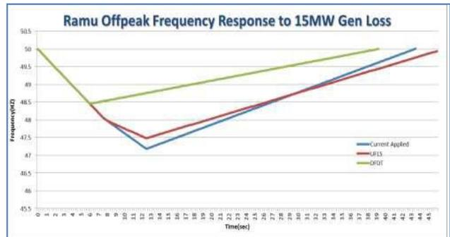
Figure 11 ROCOF for off peak load, Loss of Ramu1 Unit
