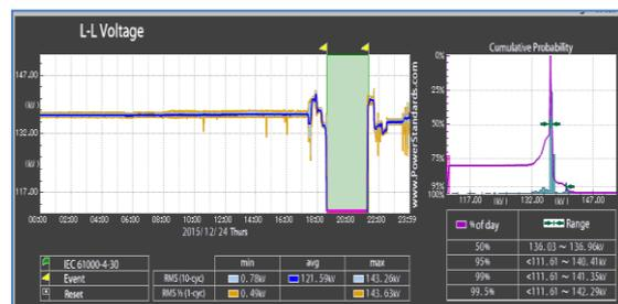
Figure 16 Voltage profile of L601 after an outage event 24/12/15
