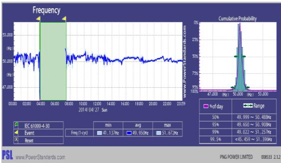
Figure 7 Ramu System frequency degradation 27/04/2014
