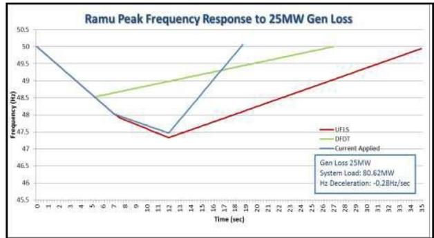
Figure 10 ROCOF for peak load, Loss of Lae TM2500GT
