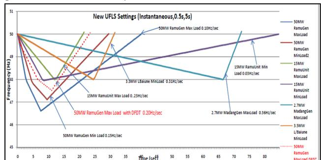
Figure 12 Frequency response of Ramu system with respect to loss of generation
