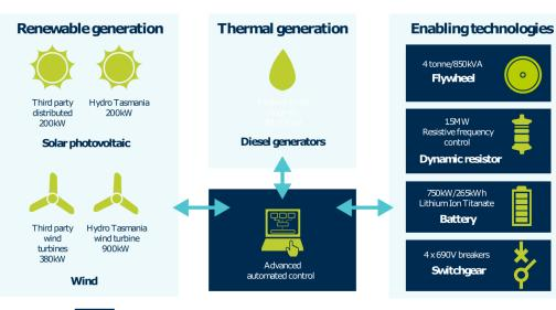
Scalable modular systems capable of low cost rapid deployment
