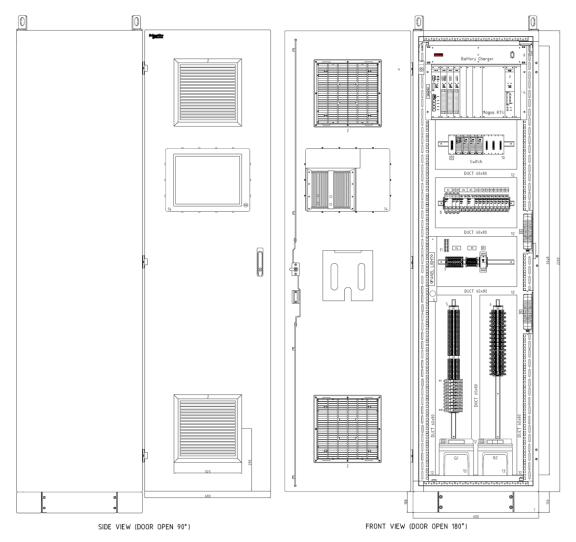
ExampletypicalSCADA panel general arrangement drawing shown below:
