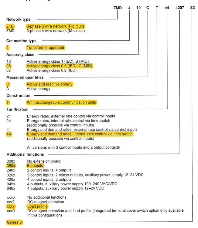
As the communication unit is a device on its own, it is not part of the meter's type designation. The customer can exchange it at any time without opening the certification seal. Each communication unit has its own user manual.
