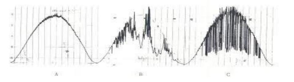
Rules of thumb exist for the allowable percentage of solar generation to maintain grid stability. They vary according to the distribution of the solar generation With one large solar farm and little other solar, about 20% of the noon time load can come from solar without stability issues With two or three widely separated large solar farms of roughly equal size (more than 5 km separation) 30% to 40% of the noon time load can generally come from solar without stability issues
