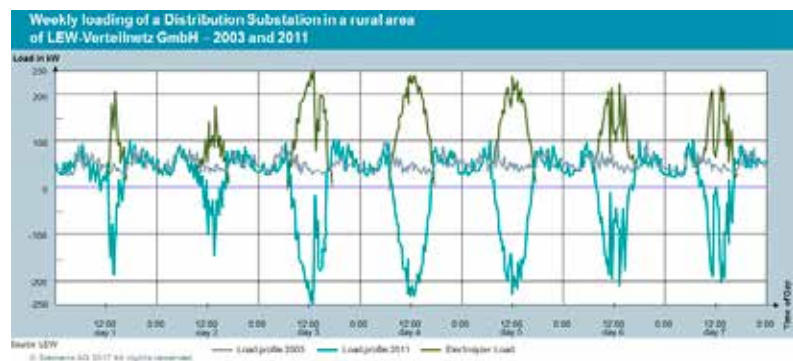
Figure 10 - Load profile for distribution substation with Silyzer Implemented
