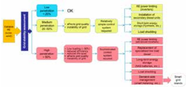
Figure 3 - PV Integration strategy based on level of PV Penetration [4]
