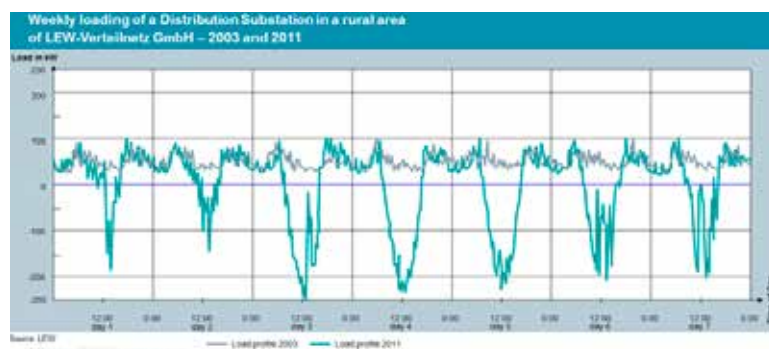
Figure 2 - Weekly loading of a Distribution Substation - before and after the installation of High Penetration PV
