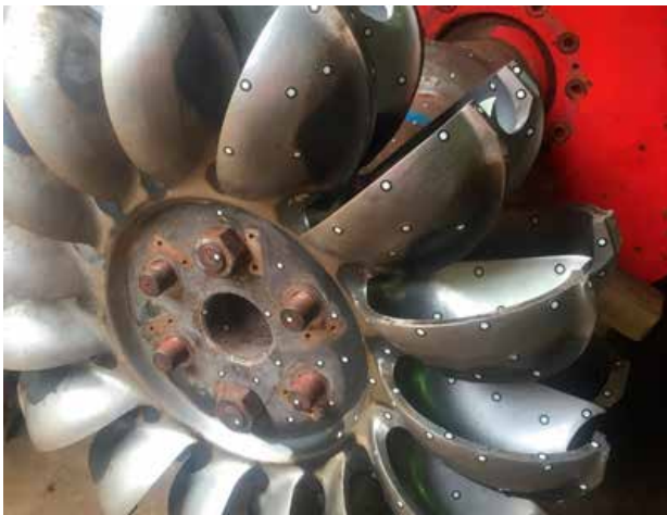
Figure 2: Pelton wheel covered with reflective targets ready to be scanned.
