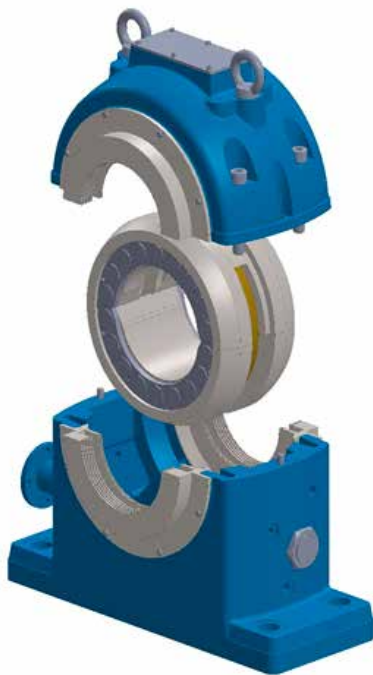
Figure 5: Exploded view of bearing assembly.
