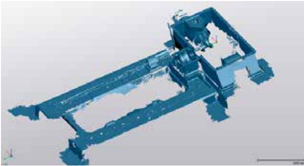
Figure 4: 3D scan of the generator bed with surrounding equipment.
