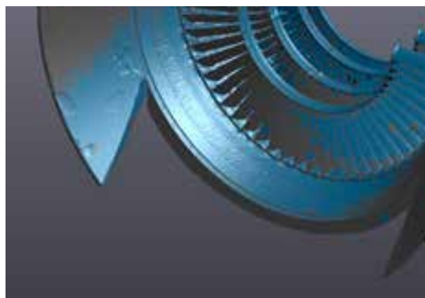
Figure 10: Two aligned scans of a gas turbine diaphragm.
