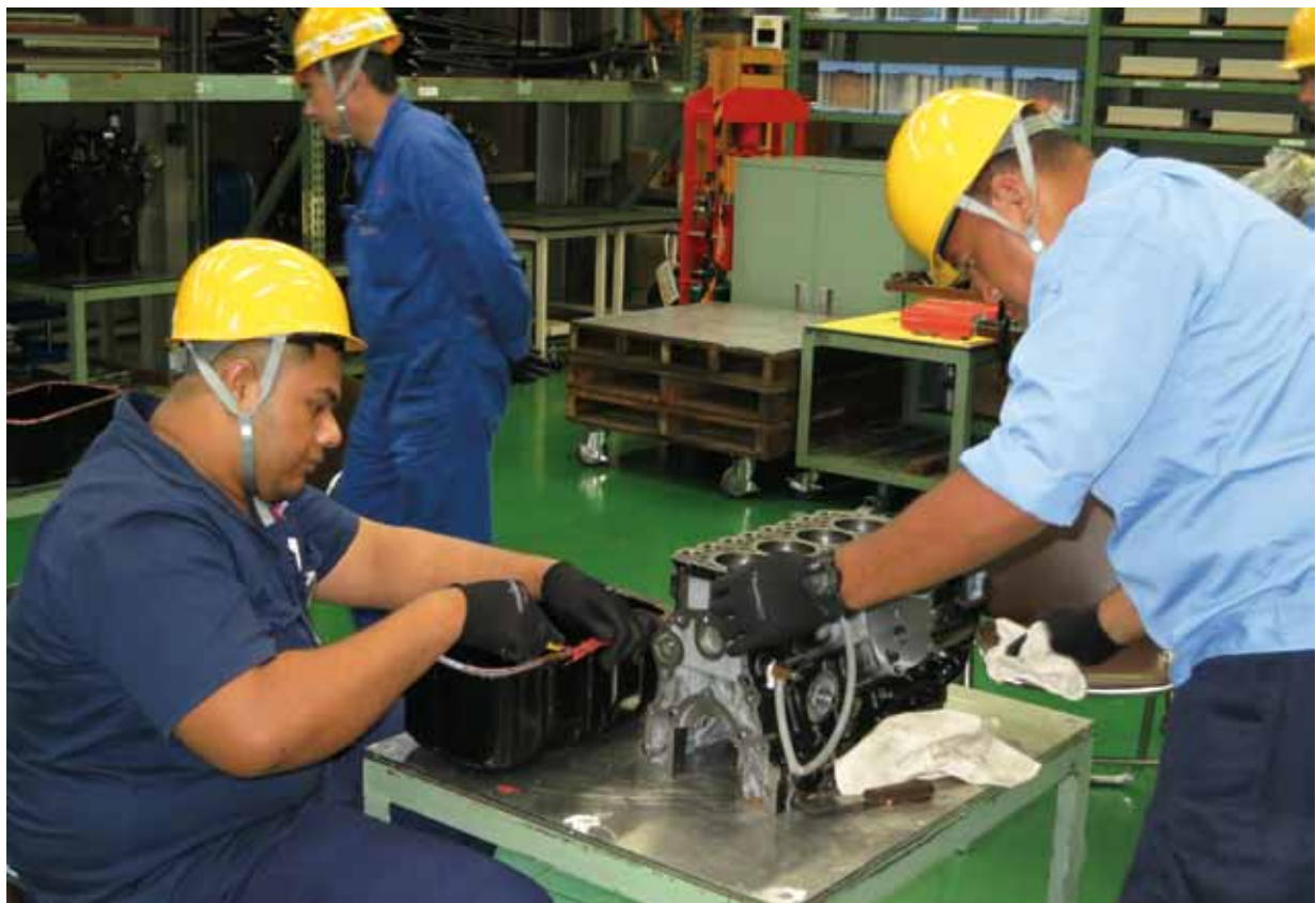
PIF Participants Training on Engine Disassembling
