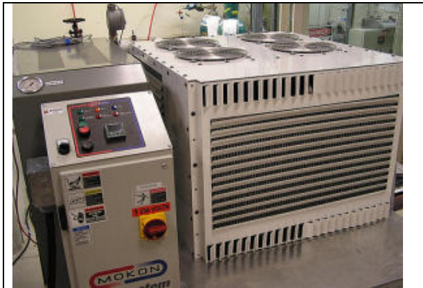
Thermal activated cooling system. This prototype of a "thermal activated cooling system" has been developed by engineers at Oregon State University, and promises important new advances in energy efficiency by using wasted heat. (Credit: Photo Oregon State University)
